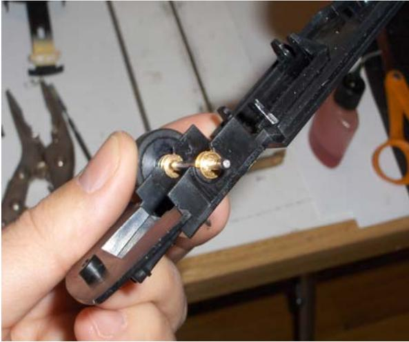
The axle should feel very tight spinning but you should be able to turn the axle. If the axle binds, the super glue can be removed by scraping it with a hobby knife. Start the process over again until you get it right. Perform this for both bushings.
