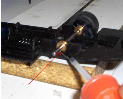
Glue your bushings to the chassis. I use super glue. Put some on the bottom of the bushing. If you ever have to remove the bushings, you can cut the glue with a razor knife.
