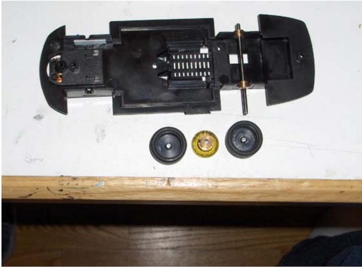
Your next step is to install your rear tires and gear. I highly recommend using Slot It rims as they are true and you have a wide selection of tires and sizes to use. I also recommend using only Slot It S1 or PPR tires as they seem to have the most grip for both wood and plastic tracks. Please note if you are using a sidewinder, you should purchase the taller rims to make sure you have enough clearance for the gear.
