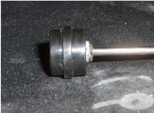
Take the front tire off the rim and inspect for smoothness. There should be no flashing or any rough spots that would cause tire to be out of round. If there are any rough spots, sand down the rim by putting the rims on an axle and use a dremmel at low speed. Make sure the sand paper is flat.
