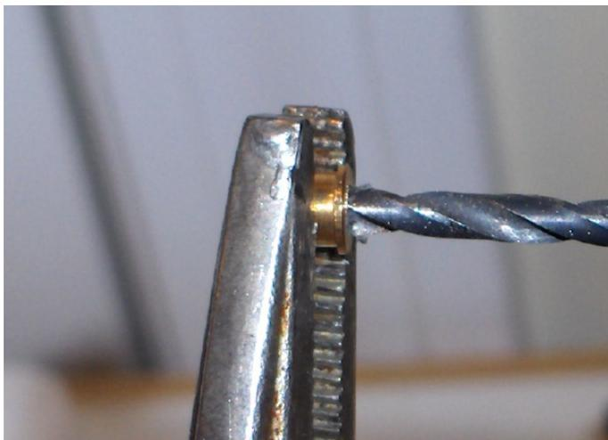
Next, move to the rear bushings. Use brass bushing as these have the best fit to the axle and the smallest amount of play. I recommend drilling part of the bushing out.
